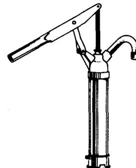
**11230 Heavy-Duty Lever Action Barrel Pump**
