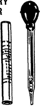
Easy to check. Floating balls indicate battery condition. Tests cars, trucks, motorcycles, and marine batteries.
