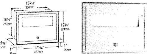
Satin-finish stainless steel. Seamless beveled flange. Capacity: 500 toilet seat covers. Rough Wall Opening: 15 3/16" W, 11 1/4" H, 2 5/8" min. depth.
