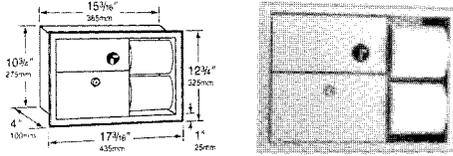
Satin-finish stainless steel. Disposal door is self-closing. Receptacle retained in cabinet by tumbler lock. Capacity: 3/4 gal. (2.8 L). Rough Wall Opening: 15 3/16" W, 11 1/4" H, 4" min. depth.
