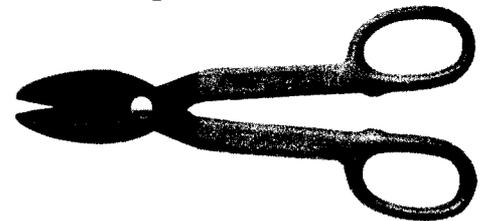
Straight pattern snips are primarily for straight cuts, although they will cut wide curves when trimming light stock. The inside edge of the blade face is flat and tends to guide the tool along a straight line. This most traditional of tinner's snips is still widely used in the plumbing, heating, air conditioning and roofing trades.
