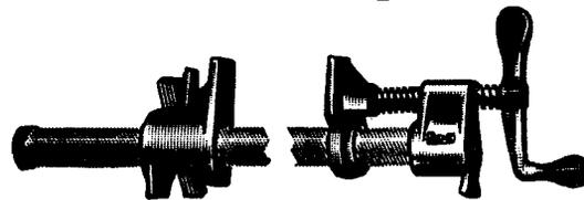
Fixtures to be used on ordinary ¾-inch black pipe as the bar. No holes, notches or rivets required to assemble; just screw the head on regular pipe threads. The foot has a multiple disc clutch which grips the bar automatically at any point. Most rapid action, secure holding power and easy release. Hardened clutch disc. ¼-inch diameter screw. Clamp faces 1¾-inches square. Baked enamel finish. One "Set" makes one clamp.
