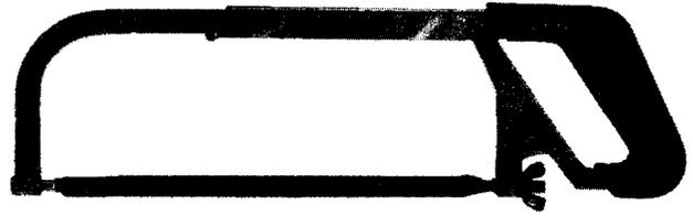
Rigid steel frame with molded cushion grip rubber handle. D-shape guard protects hand and knuckles. Frame is adjustable for 8" (205 mm), 10" (255 mm) and 12" (305 mm) blades, allows blade to be faced in four directions. Furnished with 10" 255 mm standard carbon steel blade.
