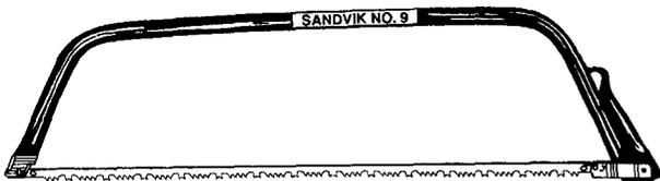
Lightweight all-around saw for pruning, gardening, farming and construction work. The 9 bowsaw features a tubular steel frame and steel plate tension lever. Replaceable Sandvik 51 hardpoint blade with peg tooth pattern for smooth cuts in green and dry wood. Available on 9-21 inch and 9-24 inch bowsaws. The Sandvik 23 hardpoint blade with raker tooth pattern for cutting green wood. Available on 9-30 inch and 9-36 inch bowsaws. All 9 bowsaws come with knuckle guard and plastic sheath for blade.
