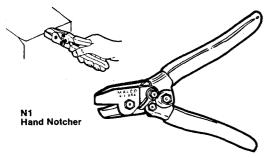
Fast and easy cutting. Notcher makes a clean 30° "V" shaped cut in sheet metal. 13/16" maximum throat depth. Upper cutting jaw is drop forged high impact alloy steel. Hook design of cutting jaw facilitates notching corners or take-off tabs to desired depth without slipping. Nickel plate and black oxide finish. Blue grips.
