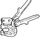
Compound leverage increases mechanical advantage nearly 7 to 1. Simply squeeze handles together with one hand while holding stud in place. A unique punch and die shape creates a rectangular crimp, bending over thicknesses of channel and stud at the same time to form a sturdy bond.
