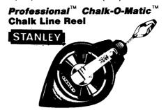
Die cast case. Felt gasket hugs line, distributes uniform chalk coating. Universal hook attaches to any projection or slot. Can be used as plumb bob.
