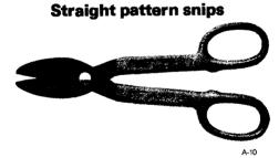
Straight pattern snips are primarily for straight cuts, although they will cut wide curves when trimming light stock. The inside edge of the blade face is flat and tends to guide the tool along a straight line. This most traditional of tinner's snips is still widely used in the plumbing, heating, air conditioning and roofing trades,
