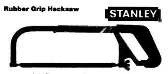
Rigid steel frame with molded cushion grip rubber handle. D-shape guard protects hand and knuckles. Frame is adjustable for 8" (205 mm), 10" (255 mm) and 12" (305 mm) blades, allows blade to be faced in four directions. Furnished with 10" 255 mm standard carbon steel blade.
